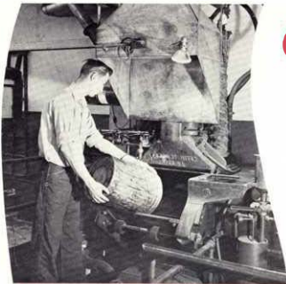
The operator is dumping carbon black into one of the Banbury mixers, ventilated by our Dustube.
