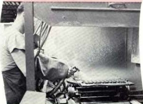
A rubber mold being cleaned in the No. 64 Liqueamette. The side door, normally closed, is open to make possible the picture.
